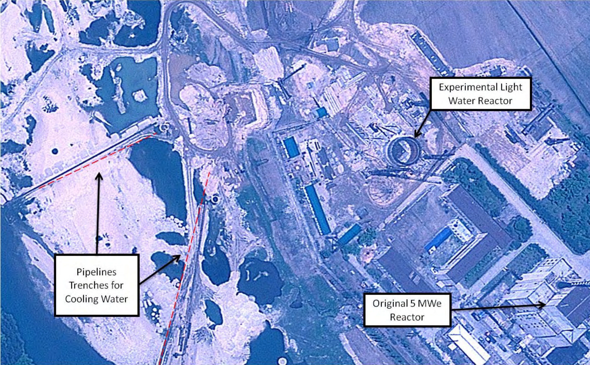
Figure 3. By May 22, 2011, in addition to further construction progress, there are pipe traces to the river for supplying cooling water and hot water discharge. Image Credit: Includes GeoEye-1 and/or IKONOS Products © GeoEye, distributed by e-GEOS.
