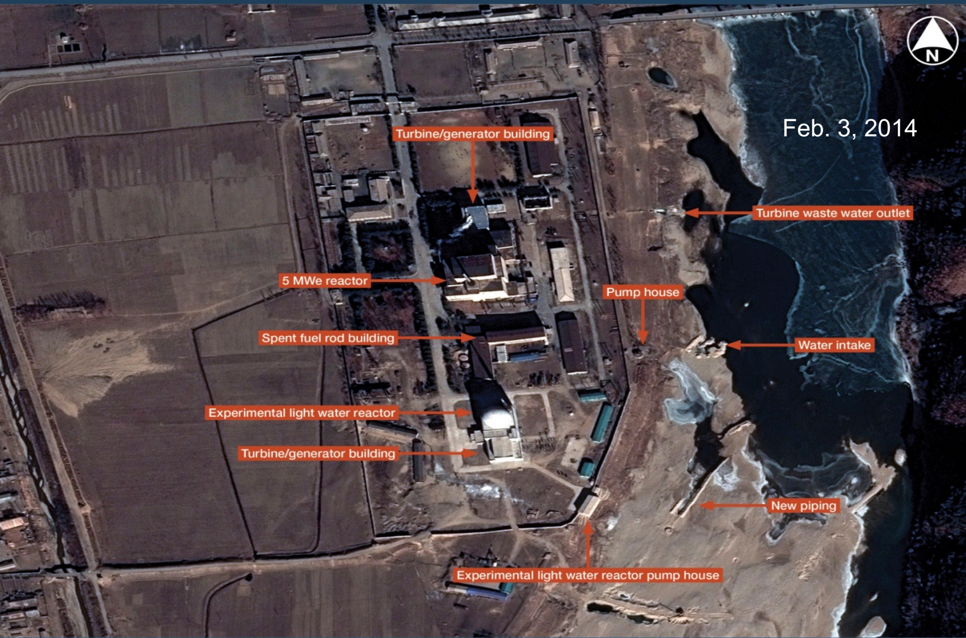
The new Experimental Light Water Reactor (ELWR) sits on the site of the original 5 MWe reactor's cooling tower. The ELWR's pump house will now serve a secondary cooling system for each reactor.
