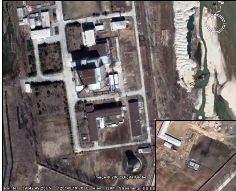
5 MWe reactor Shut down. Capable of 6 kg Pu per year. (No cooling tower)
