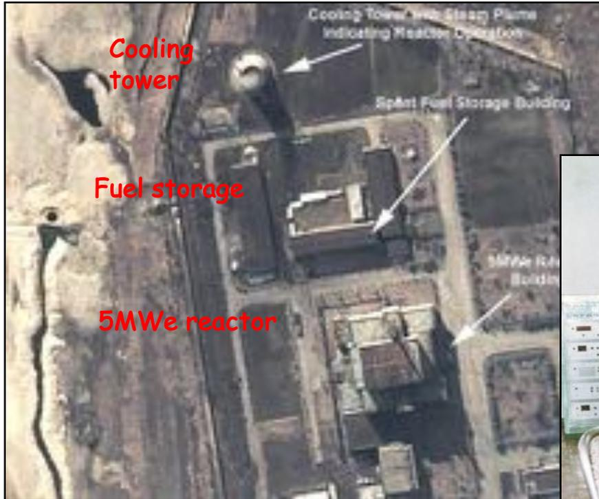
Reactor is providing heat and electricity for town ...
