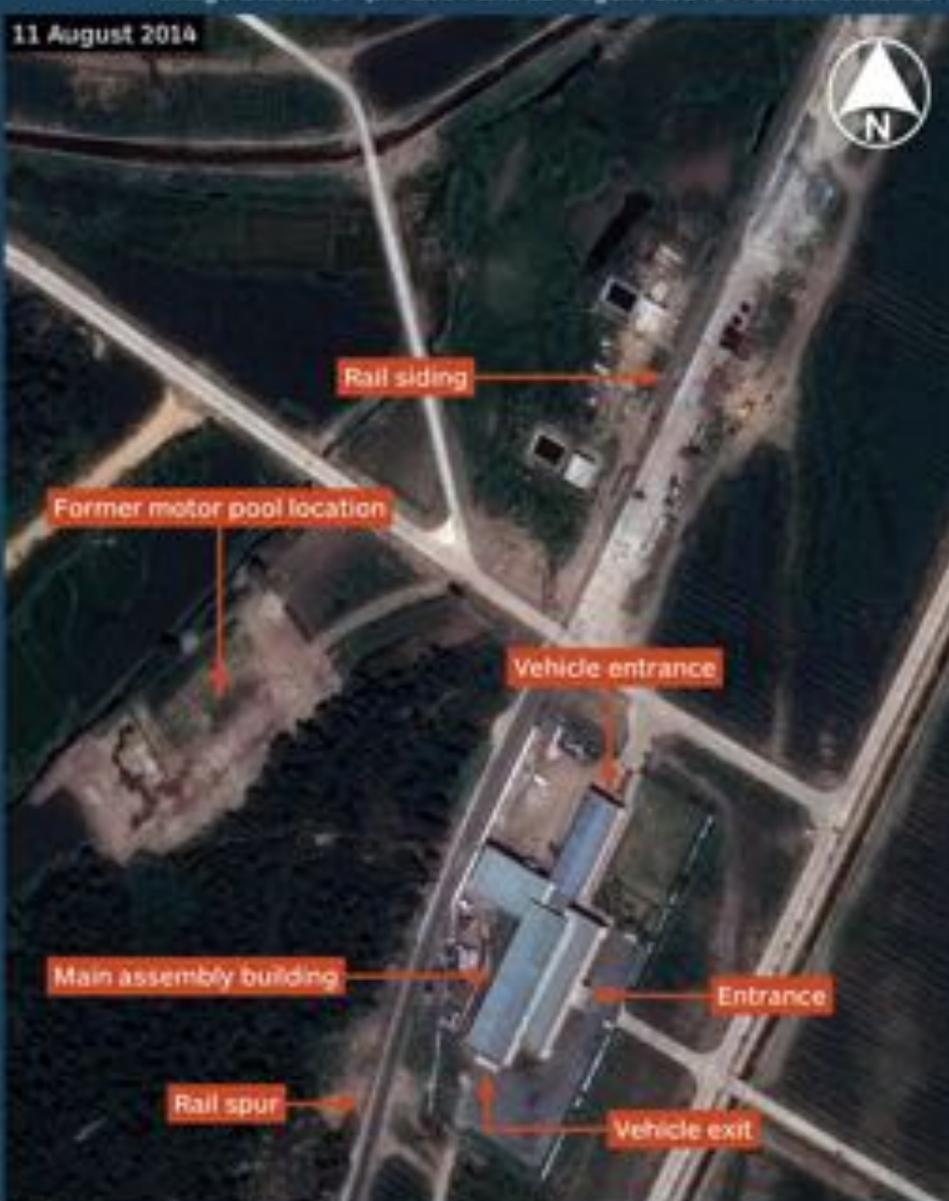
Airbus Defence and Space imagery shows infrastructure changes around the Sohae horizontal assembly building. During 2014 the rail spur, previously terminating at the rail siding, was extended to provide direct access to the launch pad.
