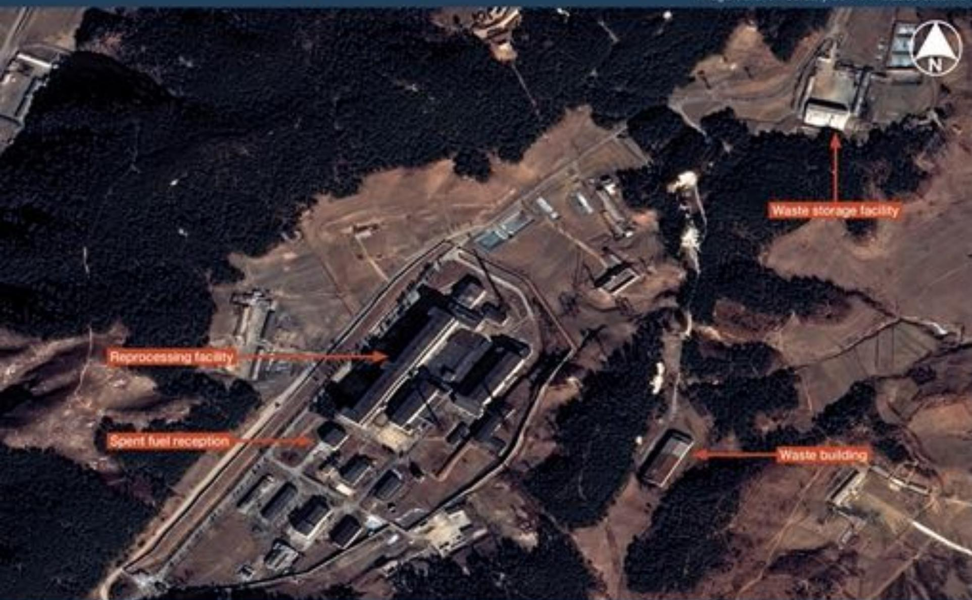
The Plutonium separation facility was the last of the major facilities completed in the southern area. Here spent fuel is processed to extract its plutonium. Although no plutonium has been processed here since late 2009, the facility has been kept in a standby condition and should be ready to process the fuel rods currently in the 5 MWe reactor, expected in about a year.
