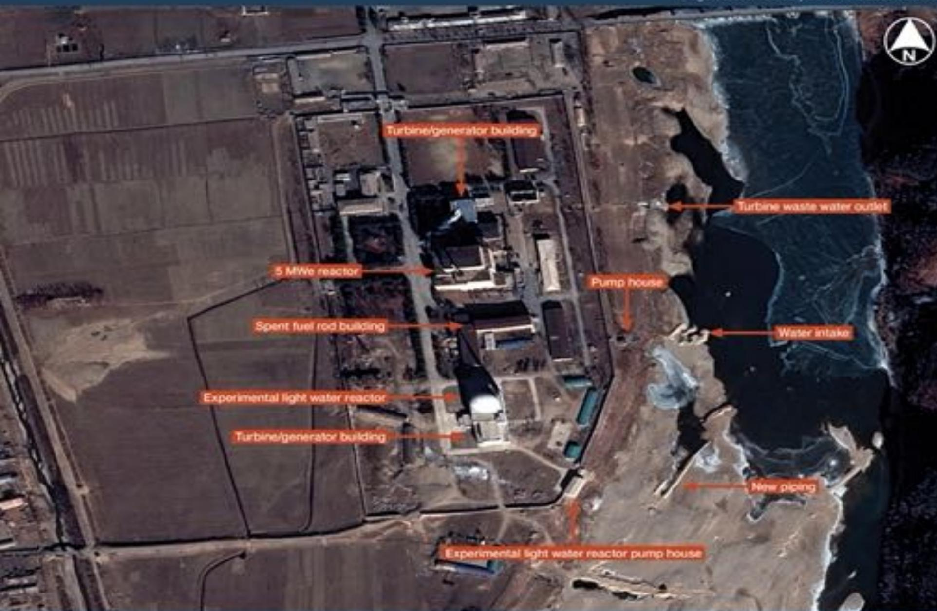
The new Experimental Light Water Reactor (ELWR) sits on the site of the original 5 MWe reactor's cooling tower. The ELWR's pump house will now serve a secondary cooling system for each reactor.
