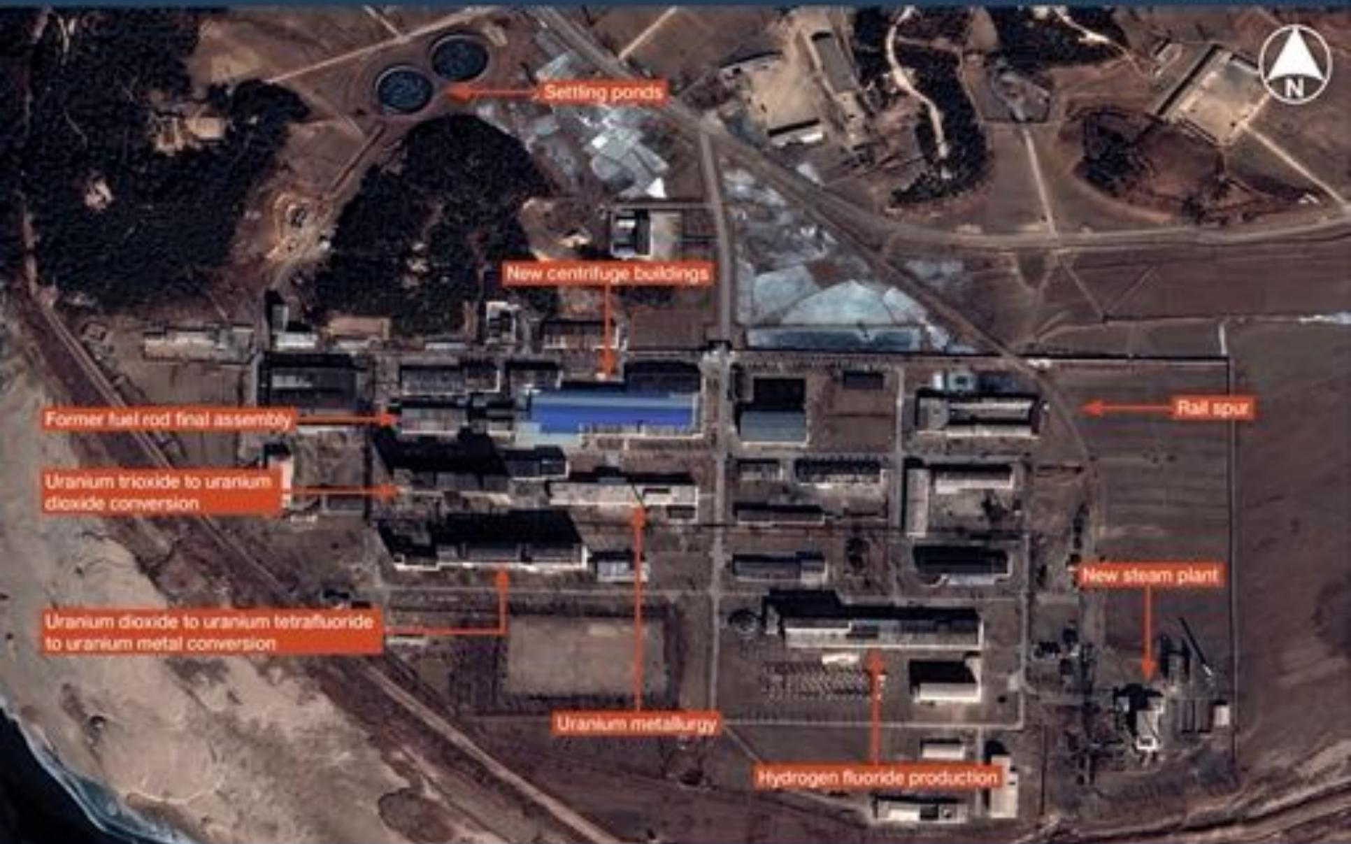
The fuel fabrication facility is the largest of the functional areas in the southern half of the Centre. Visible is a new centrifuge building with an expected capacity of 2,000 centrifuges.
