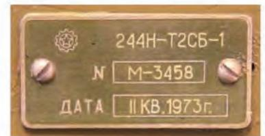
▲ The 244N bomb data table. 244N-T2SB-1 means that the bomb was assembled by the 2nd team's 1st shift. The M-3458 is its serial number. The II KB. 1973g means that it was assembled in the 2nd quarter, in the year of 1973. Vladimir Astalkovits
