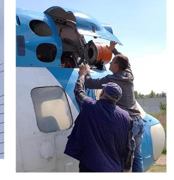
Fig 1, 2 & 3 Helicopters with Sr(Y)-90 "BIS-1" sources
