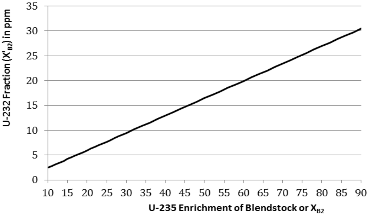
Figure 4: U-232 fraction expressed in ppm in the blendstock as a function of the blendstock U-235 enrichment.
