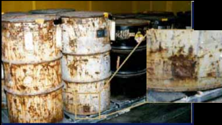
The past: corroded HEU drums, Y-12 Building 9206
